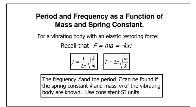
Example 2: The frictionless system shown below has a 2-kg mass attached to a spring (k = 400 N/m). The mass is displaced a distance of 20 cm to the right and released. What is the frequency of the motion?
