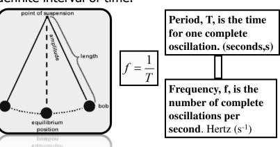
Example 1: The pendulum makes 30 complete oscillations in 15 s. What is the period and frequency of the motion?
