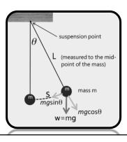
A <u>restoring force</u>, F, acts in the direction opposite the displacement of the oscillating body.
