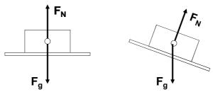
On a flat surface, the normal force, F<sub>N</sub>, is equal to weight of the object.
